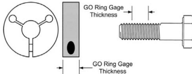
Sometimes when threads do not assemble smoothly it is appropriate to measure the thread's pitch to determine if it is within the allowable variation. The thread's pitch is the distance between the same location on two adjacent threads measured parallel to the thread's axis. Most of the time when dealing with threads the terms lead and pitch are used interchangeably. The pitch length is equal to one divided by the number of threads per inch.
